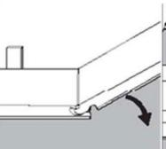
Step 2: Lock short end of plank by Step 3: Use leftover plank from inserting tongue into groove at an angle and drop in place. Continue to end of first row.
