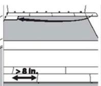
first row as starter for second row. Minimum 8" stagger between plank end joints.
