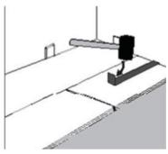
Step 8: Use hammer and pull bar to engage final piece, insert spacers and continue to next row.
